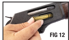
FIG 12 Firearm being loaded through the loading port
