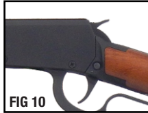
FIG 10 Hammer in the safety (half cocked) position
